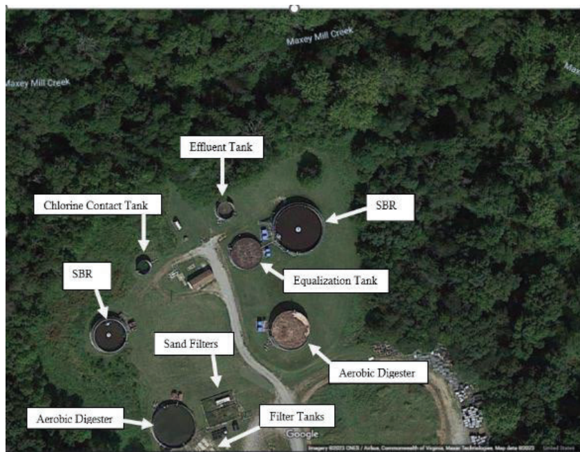
Photograph 3. Marked Aerial photograph of the Cumberland Facility's wastewater treatment plant and Maxey Mill Creek. (Source: Google Maps, modified).
